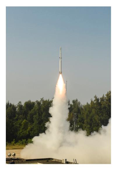
The AD-1 is a long-range interceptor missile designed for both low exo-atmospheric and endo-atmospheric interception of long-range ballistic missiles as well as aircraft. It is propelled by a two-stage solid motor and equipped with indigenously-developed advanced control system, navigation and guidance algorithm to precisely guide the vehicle to the target.
